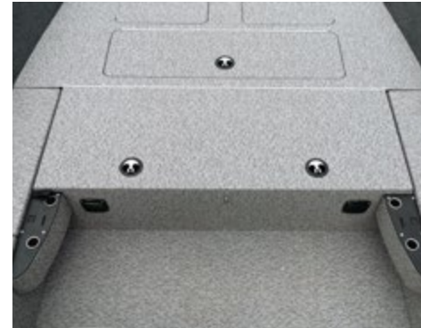
Additional locker for installing electric motor batteries and storing canvas enclosure.
