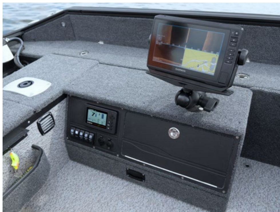
On command console 12" i 16" echo sounders can be mounted.
