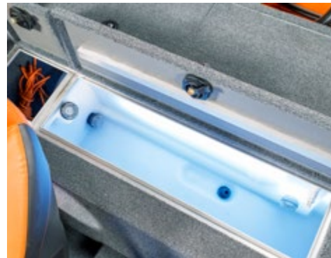
Double-circuit illuminated livewell in the aft deck
