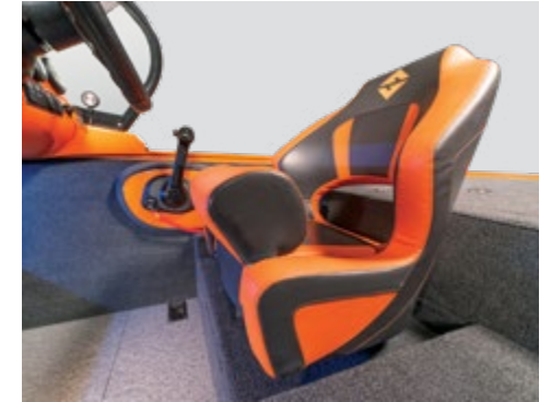
Seat with a lifting roller for easy control of the boat while standing.
