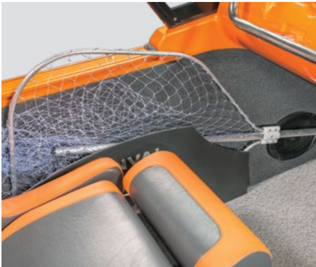
Double-circuit plastic self-filling illuminated 110 liter livewell in the aft deck
