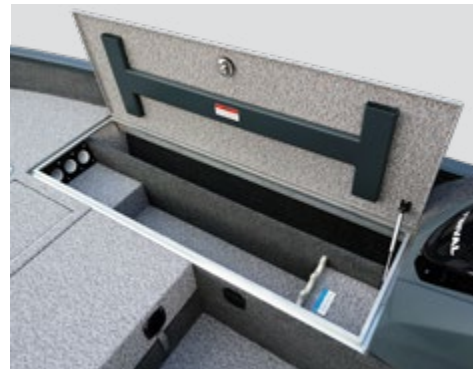
Locker for 3 rods up to 2.45 m long with storage space for the canvas enclosure.
