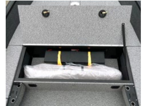
Additional locker for installing electric motor batteries and storing canvas enclosure.
