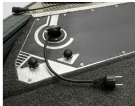
Charging batteries and controlling the trim of the engine* from the bow deck.
