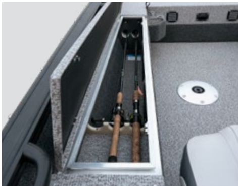
Storage for rods up to 3 m long along the port.
