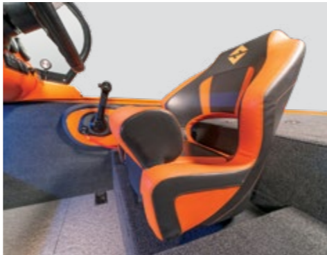
Seat with a lifting roller for easy control of the boat while standing.
