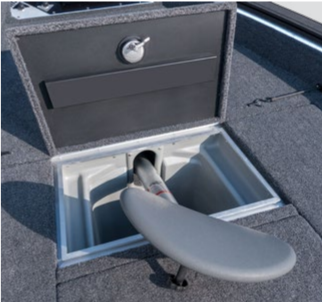
The fishing seat pedestal does not occupy extra space and is hidden in a special tunnel.
