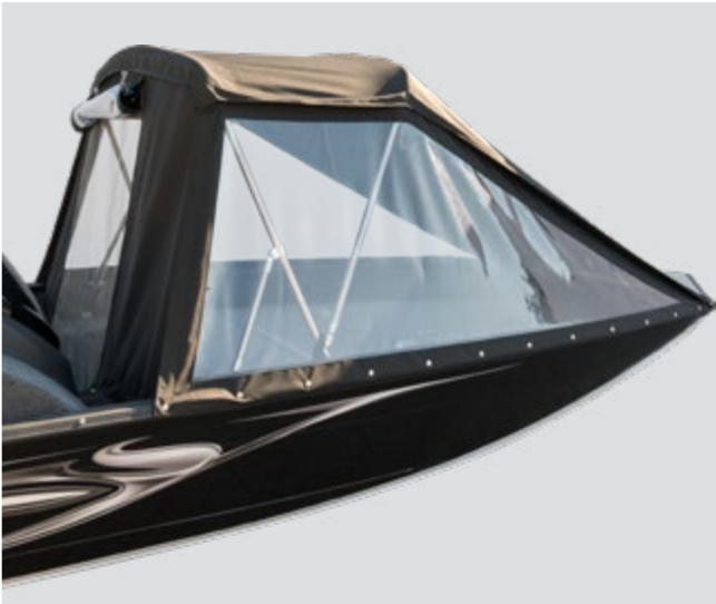
Removable side and front curtains made of transparent PVC film.
