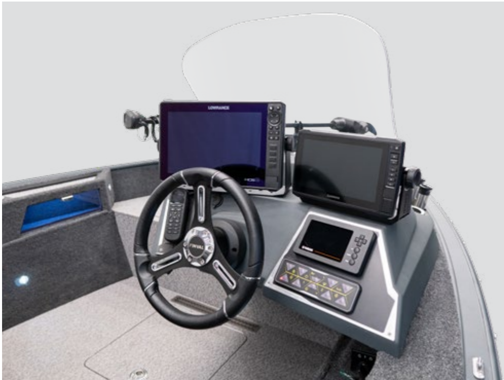
The new console is decorated with plates of anodized aluminium and makes it possible to install two 12" echo sounders.
