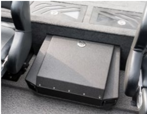
Section between seats for installation of 3 traction batteries.*
