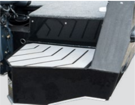
Transom extension platforms to improve stability and provide easy access to water.
