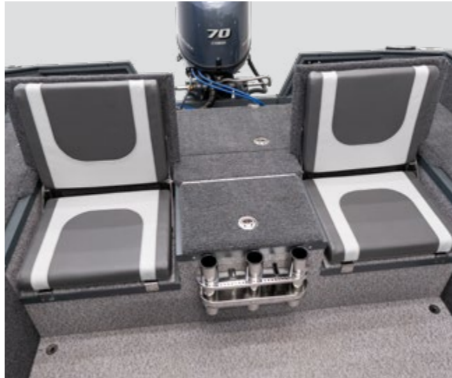
The passenger glove compartment with two compartments for things and baits, a cup holder, and a place for storage of fishing tools.
