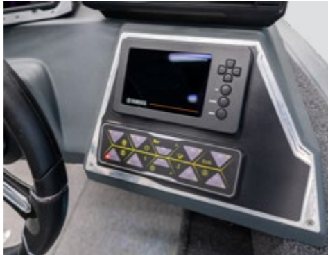
The waterproof control panel of the electrical equipment.
