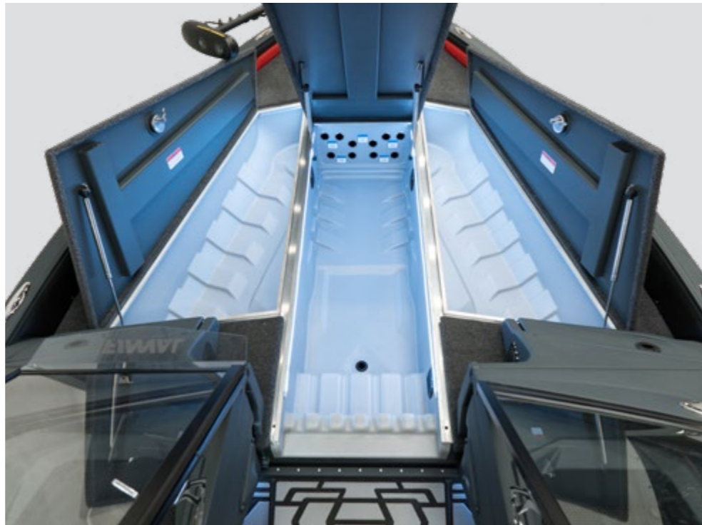
The bow deck has 2 storage compartments with a capacity of 120 liters each and a locker for 10 fishing rods. All lockers are equipped with a forced ventilation system.
