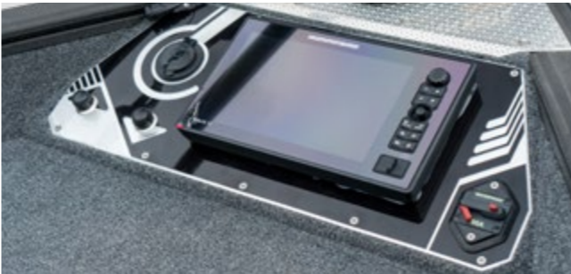
Decorative plates of anodized aluminium on consoles and a bow deck.
