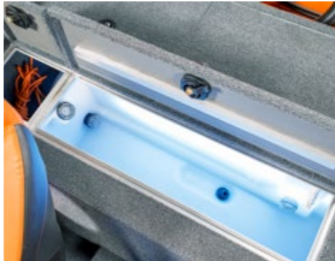
Double-circuit illuminated livewell in the aft deck
