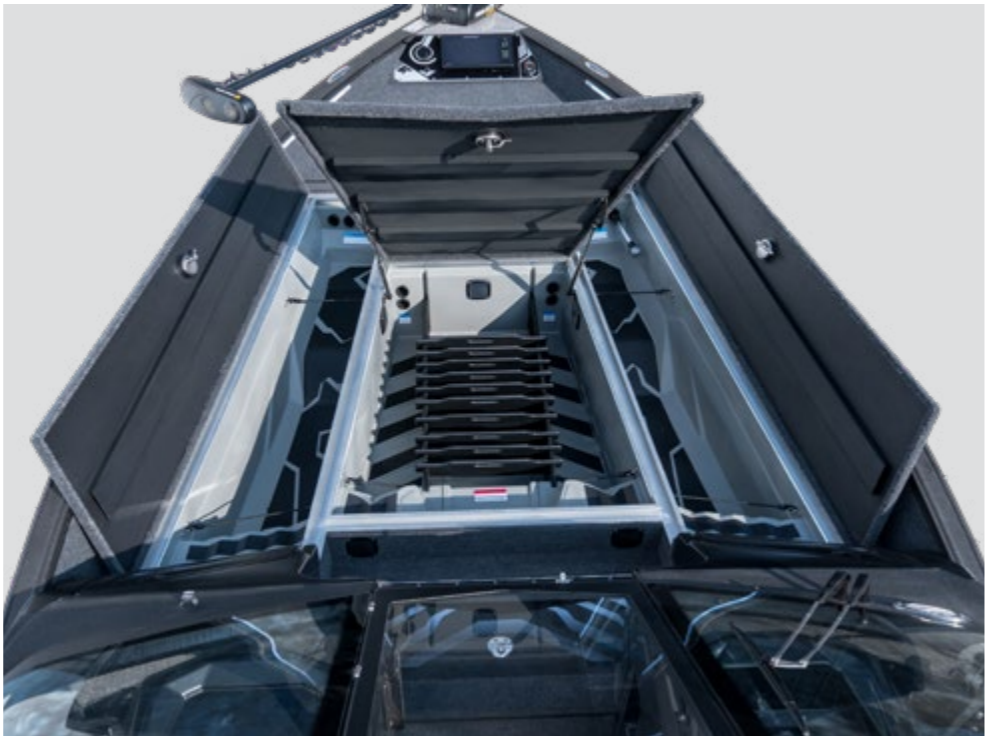
3 lockers each accommodating 4 rods with a forced ventilation system. Central locker with a capacity of 194 liters with storage space for personal items and fishing tackle.
