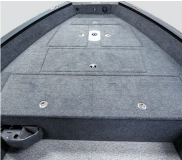
Option B of the bow deck configuration - a big locker with two hatches.
