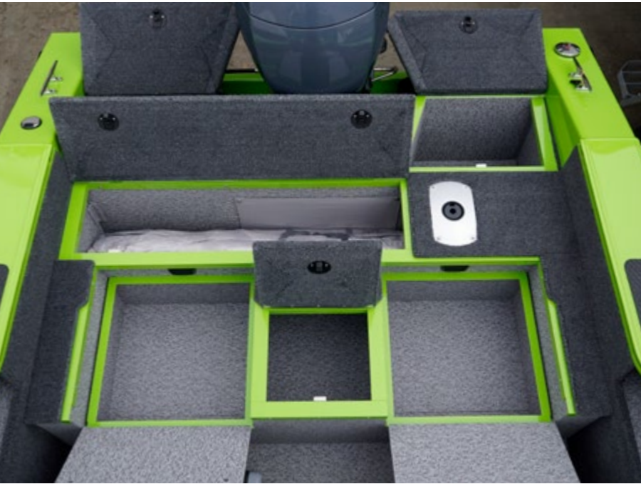
Configuration JS has a large number of stern deck lockers with a total volume of 290 liters.
